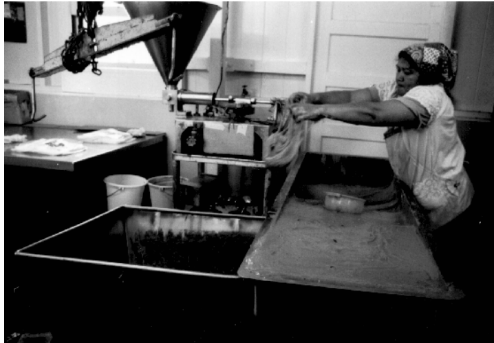
Figure 25. Strained poi in stainless steel trough being mixed before packaging (photograph courtesy of the Center for Oral History, University of Hawai'i at Mānoa).
