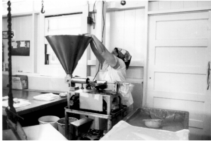
Figure 27. Poi packaging machine (photograph courtesy of the Center for Oral History, University of Hawai'i at Mānoa).
